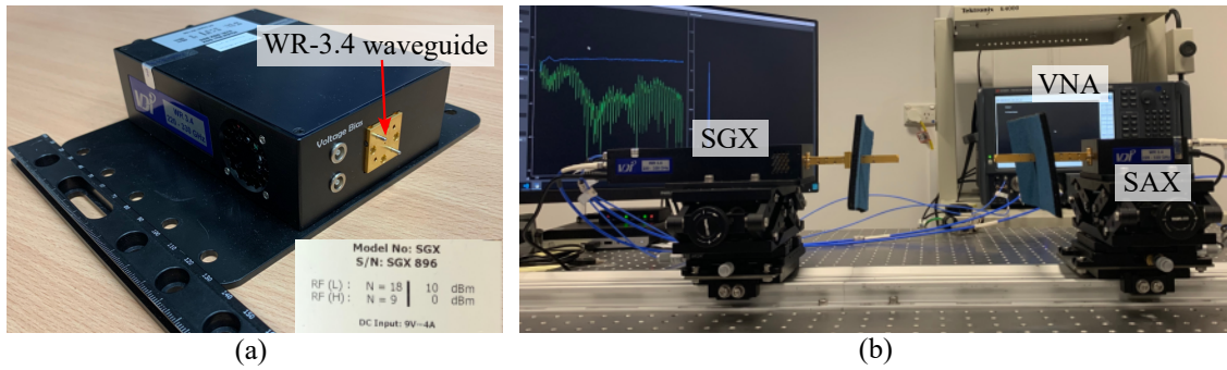
Figure 1.5. Harmonic-based terahertz source. (a) VDI signal generator extension (SGX) module. The SGX has the function of multiplying the input RF signal frequency to the terahertz range by a factor of 9 or 18. (b) A typical terahertz measurement environment at the Terahertz Engineering Laboratory, the University of Adelaide. The SGX on the left-hand side up-converts the RF signal from the VNA to the WR-3.4 frequency band, and the signal analyzer extension (SAX) module on the right-hand side down-converts the terahertz signals back to RF for characterization using the VNA.
